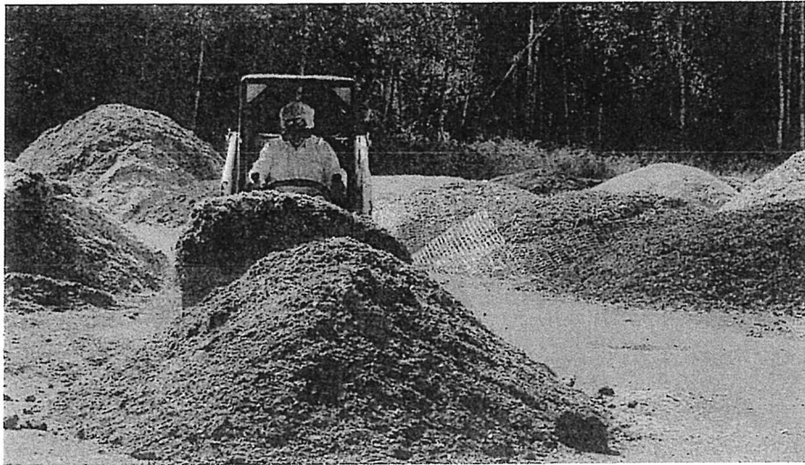
Photo 10. Skid loader turning compost pile (photo by Gary Flory)
